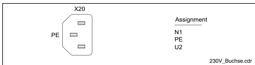
Fig. 7-15: Pin assignment of the 230/115 VAC connection X20
